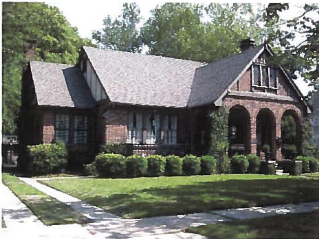
This house is an example of logical massing. There is a clear hierarchy from the primary to secondary massing that reduces the scale of the overall building in an organized fashion.
